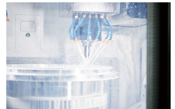
Cutting fluid being applied all around the tool during cutting
